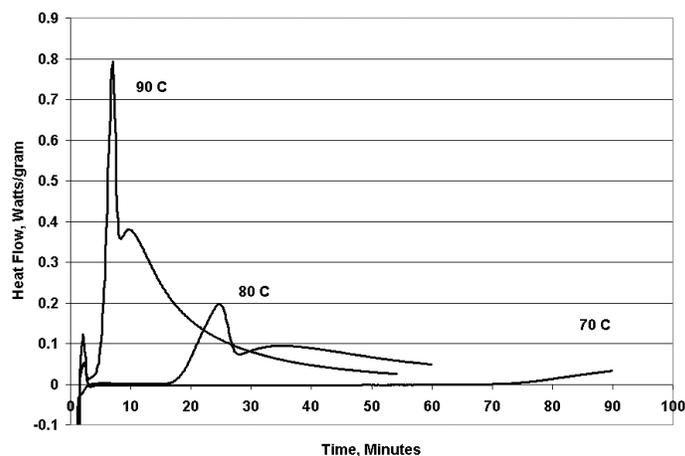
**Figure 2.** Isothermal DSC Plots (Catalyst: 1-wt.% Qsalt TRS, Exotherm up)
