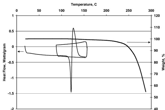
**Figure 1.** DSC & TGA Data of the Qsalt Catalyst; Heating rate: 5 °C/min (Exotherm up)
