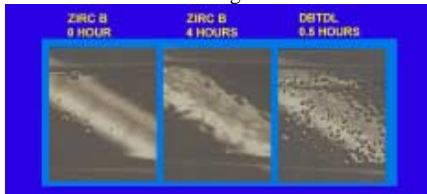
Figure 15. Film appearance of water-borne two component coating, film thickness 25 η. Cure conditions room temperature and relative humidity 50-60%. Catalyst ZIRC B and DBTDL.
