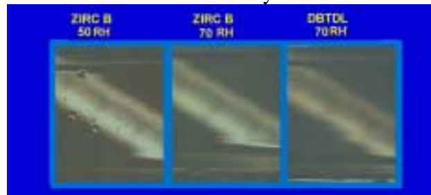
Figure 16. Film appearance water-borne two component coating, film thickness 25 η. Cure conditions, room temperature and relative humidity 50 and 70 %, ZIRC B and DBTDL catalyst.
