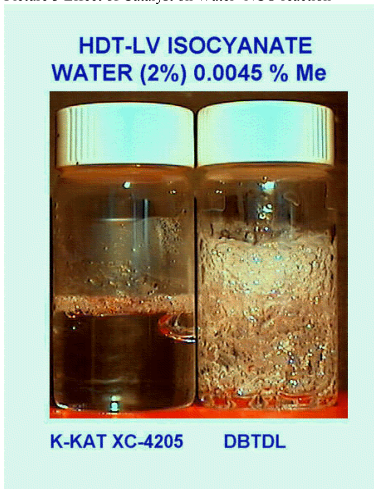
Picture 3 Effect of Catalyst on Water -NCO reaction
